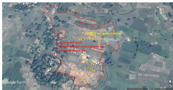
Details of the site: The red boundary is the selected site; the yellow patches indicate field bunding & LBCD and blue are proposed sites for farm pond
